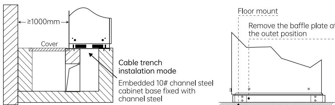
Figure 5-5 Base mounting and fixing
